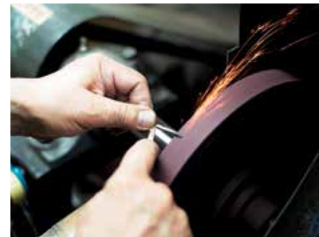
(Above) The process of installing the small edges of the make-up tools whereby each edge is grinded one by one by hand. The workmanship is important in ensuring the sharpness of the tools.
