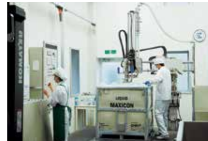
Water is packed in a new bag after each heat treatment of 120 degrees without being exposed to air.
