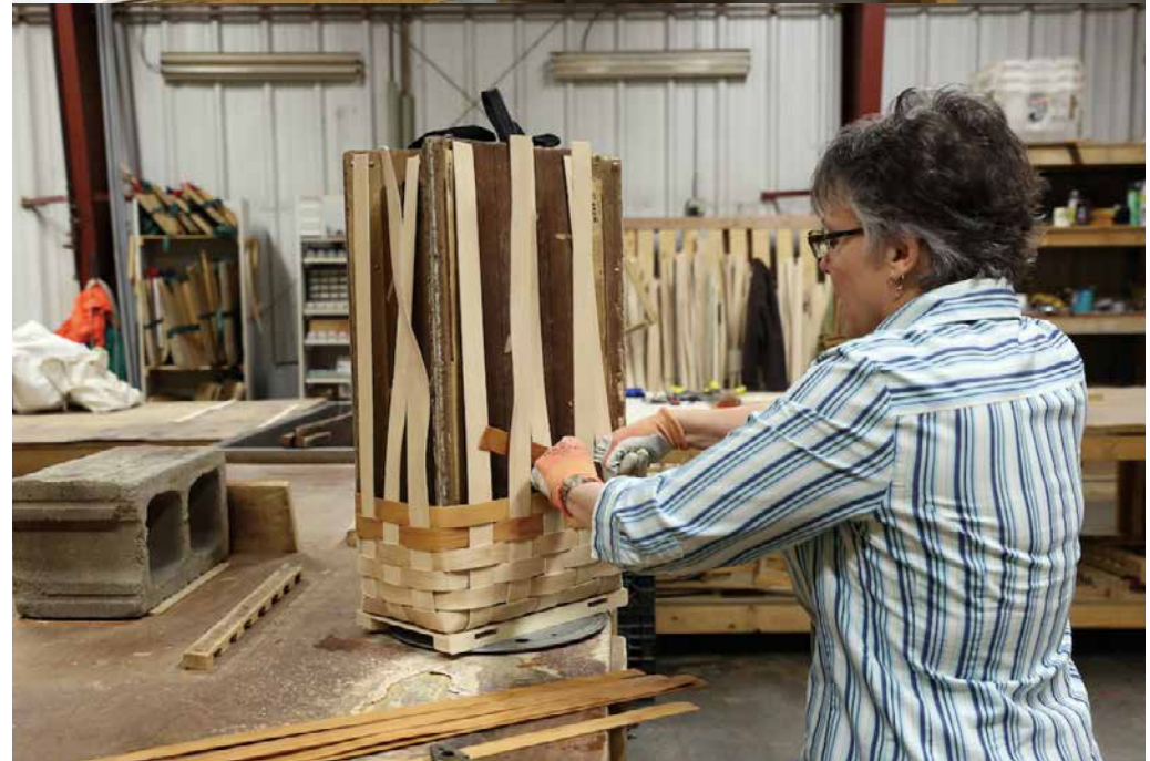
Long, thin strips of maple are soaked in water until soft. It is then fixed to the base and woven onto the frame. Once dry, the pack is surprisingly light and durable.
