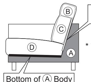
\* The frame of **B** head support is designed not to reach the bottom of **(A)** main unit.
