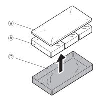
Note (Other Caution Do not open the fasteners on the non-woven fabric covers of (A) coil units and (B) cushioning material.
