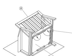
Put (b) and (c) around (a), and insert into the bolt holes on the back side of B seat (2 places). Then lightly tighten a using d to loosely attach (A) backrest.
