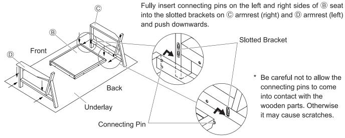
Lay 1 on its front while holding the seat with hands to prevent the connecting pins from being disengaged, and attach (a), (b) and (c).
