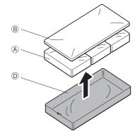
Do not open the fasteners on the non-woven fabric covers of (A) coil units and (B) cushioning material.
