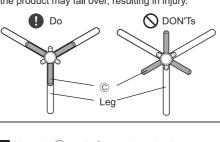
4 Attach (b) anti-slip pads to the bottoms of the legs as shown in the figure.
