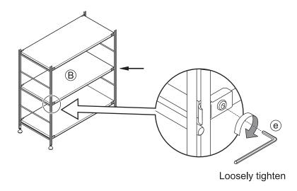
Cross the centres of the © cross bars and loosely tighten ⓑ box nut (for centre of the cross bars) and ⓐ bolt (for centre of the cross bars).
