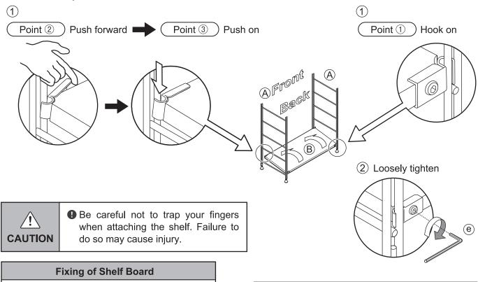
If the shelf boards are difficult to fit, gently hit the top of the shelf board so that it fits into the frame. If it still does not fit, loosen all of the hooks slightly to make it fit easily.
