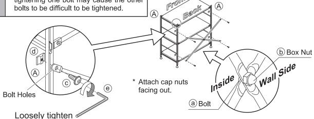
Lastly, use @ hexagonal wrench to fully tighten the hook bolts for B shelf boards that were loosely tightened in steps 3 to 5, and the cross bar and © bolts that were loosely tightened in steps 6 and 7. (17 in total)
