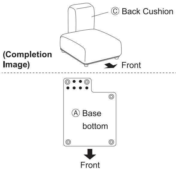
**2** Place **©** back cushion on a protective underlay with the side with label up, then place **Ⓐ** base in the direction you chose in the step **1**. Locate the bolt holes on **Ⓐ** base bottom and tighten **a** bolts for back cushion with **b** spring washer and **c** washer using **d** hexagonal wrench.
