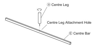
With ⓐ centre leg facing downwards, fit ⓑ centre bar into ⓑ centre bar fitting brackets attached to ⓑ headboard and ⓑ footboard.
