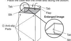
Assembling ® drawer. Fold the long-side walls up and the short-side walls inward so the corner flaps are tucked inside. Then insert the small tabs into the slits on the bottom and fit the large tabs into the recesses on the short-side walls.
