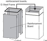
Fold the reinforcement boards and slide
