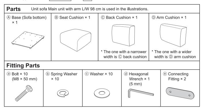
(e) Connecting fitting is a part that would be used to connect multiple units. It is not necessary when the product is used without being connected to any other unit. (See Connecting Multiple Units for details.)
