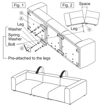
Finally, slowly raise the connected sofa units back to the upright position while holding whole units to prevent any strain on @ connecting fittings.
