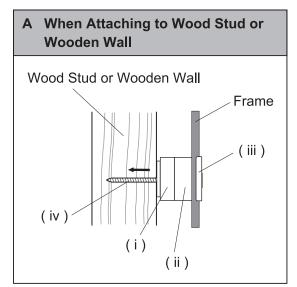
① Put ( i ) to the wall and mark the installation hole.
