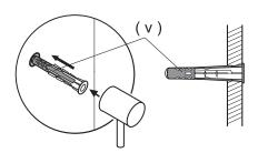
③ Set (i), (ii) and (iii) with the frame in between as shown in the illustration below, and fix the parts to (v) that has been inserted into the wall using (iv).
