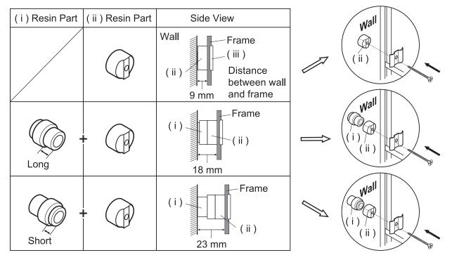
Check the wall material, and attach the parts according to any one of the procedures A, B or C.
