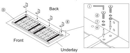
Align the holes of ® (attached in 1) with the holes of A back board, and while holding ® in place with a hand, attach © with h, and d, f, and e with i to B base. When attaching d, hold © with h.
