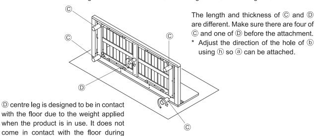
Make sure the bolts that were attached in 1 to 3 are fully tightened before bringing the sofa back upright.
