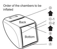
After the air chamber is fully inflated, close the lid, making sure there is no gap. Otherwise the air may leak out.
