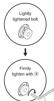
Note (Other Caution) A slight gap may be visible between (A) top board and (B) side board due to structural characteristics of the product, but this will not affect the use of the product. If there is some wobbling, loosen the bolts, and adjust the position of (A) top board and (B) side board. Then retighten the bolts.
