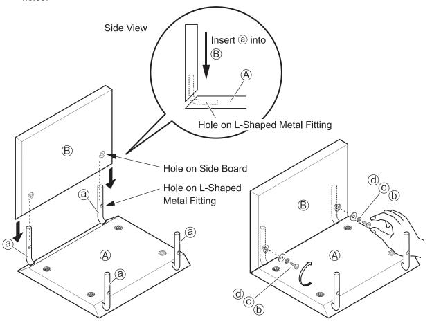
Insert a into B side board on the other side in the same way as step 3 .
