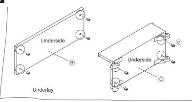
Adjust the angle of © barrel nuts with your flat-head screwdriver as shown below.
