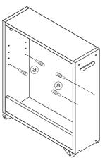
Insert ⓐ dowels firmly as they are designed to be difficult to pull out.
