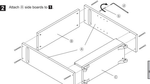
Note (Other Caution Do not tighten one bolt at a time at this point. Otherwise the positions of the holes will not be aligned, making it difficult to assemble the product.
