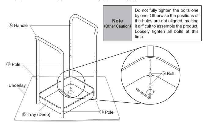
① In the same way as step ②, align the positions of the holes on ⑤ tray (deep) with the Guide Hole for Middle Tray at the desired height on ⑥ handle, and loosely tighten ⑥ bolts from the inner side of the tray using ⑧. (Eight locations in total) (The bolts will be fully tightened in step 4)
