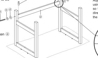
Adjust the direction of the groove using your flat head screwdriver, so the bolt hole of (b) faces the direction of a to be inserted from the side
