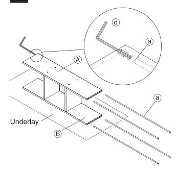
Ensure there is (A) top board on the top and (B) shelf board (with blind holes) on the bottom as shown in the illustration on the left beforehand. Then insert (a) from the right. (c) bolts tightened on (A) top board in (3) should be visible from above.
