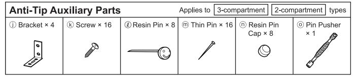
Use your own cross-head screwdriver or gimlet when attaching the anti-tip auxiliary parts.
