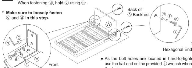
• As the bolt holes are located in hard-to-tighten areas, use the ball end on the provided (i) wrench when fastening
