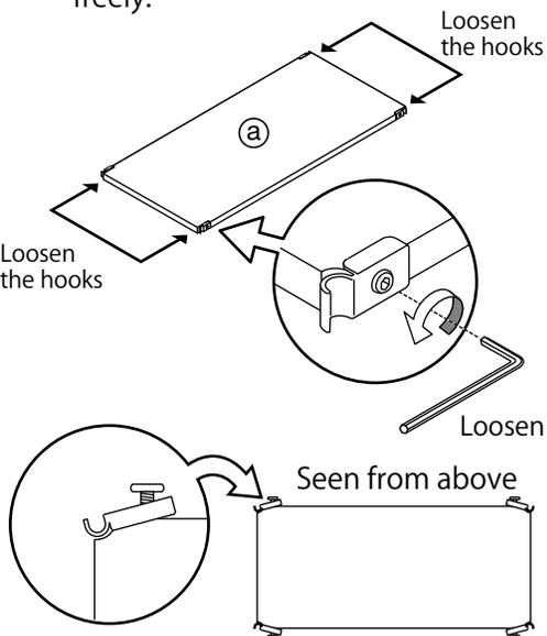
\* Loosen the screws of all the hooks of the board (as seen in the above diagram), and ensure the hooks are positioned in an inverted v shape.
