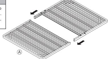
② Fix ③ C-shaped connecting parts to ④ steel frame using ③ bolts, ⑤ cap nuts, ⓒ washers and ⓓ spring washers as were in 1 - ③.
