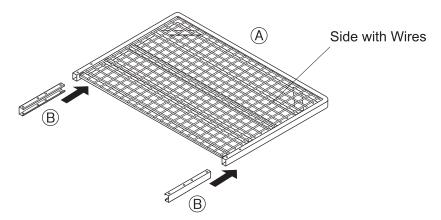
② Align the holes on ® C-shaped connecting parts and the holes on A steel frame (2 holes on each side).
