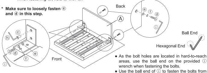
Insert ® into the holes in front of A backrest, and loosely fasten a with f and from the back of A backrest using i.
