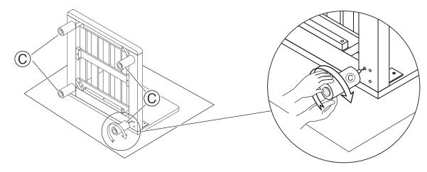
Bring the main unit to its upright position, and firmly tighten all the bolts that were loosely fastened in steps 1 to 3.
