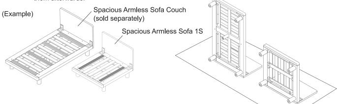
Detach legs from each product, place the connecting part, then attach the legs back again with the connecting part in between the legs and the seat frames.
