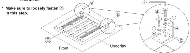
Align the holes on ® attached in 1 with the holes on A backrest, and, while holding A backrest with hands, loosely fasten © using h as well as d with f and e using to attach s to A backrest. When fastening d, hold © with h.
