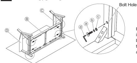
Put ⓐ through ⓑ and ⓒ, and insert into the bolt holes on both sides of ® base (4 places). Then, rightly tighten ⓐ to temporary attach ⓒ armrest (right) and ⑤ armrest (left) using ⓓ.
