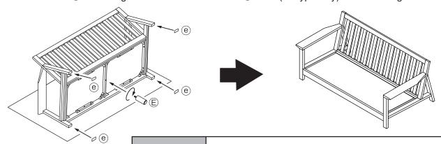
Note (Other Caution) Remove any dust and other debris from the attachment surface before attaching (e). It may not adhere well if there is anything on the surface. Press the whole pad firmly so it adheres evenly.
