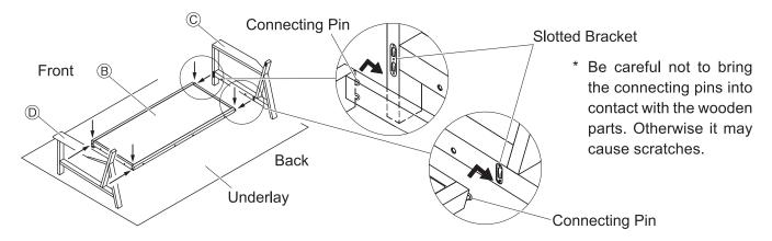
Lay 1 on its front while holding the base with hands to prevent the connecting pins from being unlatched, and attach (a), (b) and (c).
