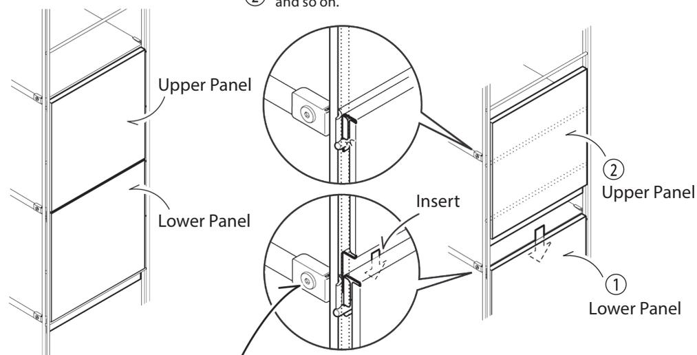
If the space between the shelf and the shelf frame is too small to fit the Side Panel slot, loosen all shelf hook screws, and then install the Side Panel.
