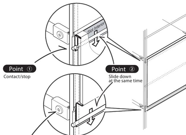
If the space between the shelf and the shelf frame is too small to fit the Side Panel slot, loosen all shelf hook screws, and then install the Side Panel.
