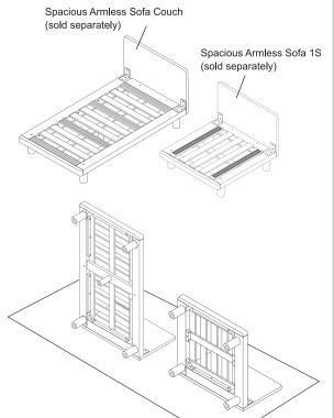
Remove the leg(s) form the area where  ${\widehat{\mathbb A}}$  connecting part is to be attached, and place  ${\widehat{\mathbb A}}$  connecting part.
