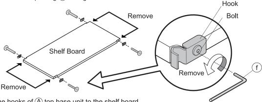
Attach the hooks of (A) top base unit to the shelf board.
