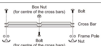
2 After attaching all shelf boards, place the frame and Ⓐ cross bars from the back in between the Ⓑ nut and Ⓒ bolt. Fasten the Ⓐ cross bars using the Ⓓ hexagonal wrench. Firmly tighten the Ⓑ box nut and Ⓒ bolt (for centre of the cross bars) using the Ⓔ hexagonal wrench.
