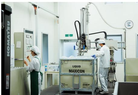
The water that is collected from the bedrock is contained in a liquid container after going through the process of filtration and thermal disinfection.
