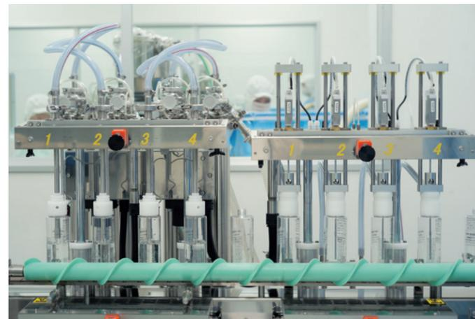
We use the machine on the right to pump clean compressed air into the lotion to air clean it then use the filling machine on the left to package the lotion.
