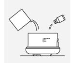
Fill the tank with essential oil and water, then place back the cover. Guideline: 7-10 drops of essential oil to 350ml of water
