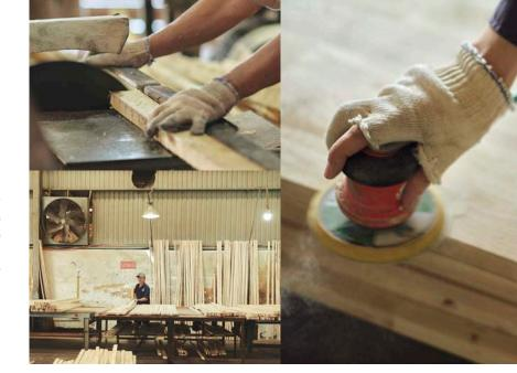
Square lumbers are joined by finger joint processing before being laminated. Small holes are covered to provide a smooth finishing before shipping out to the furniture factory.
