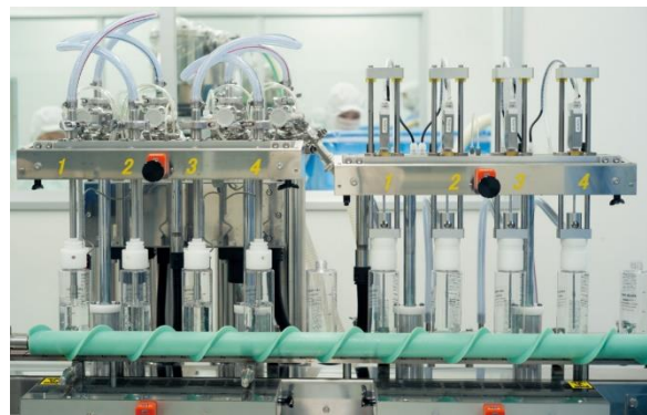
After being cleaned with compressed air in the machine on the right, bottles are filled with toning water in the machine on the left.
