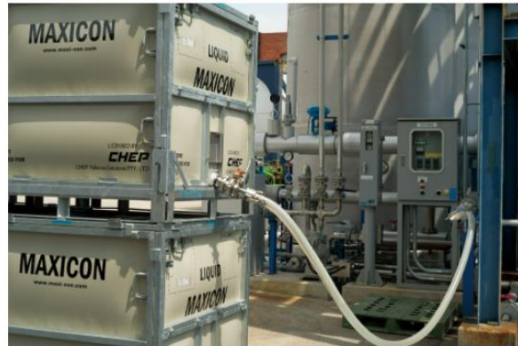
At the factory, the water is moved to the stirring tank without exposing it to the atmosphere.
