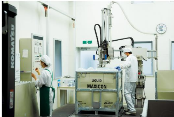
Liquid containers are filled with water collected from mountain bedrock, filtered, and thermally sterilised.
