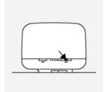
Press and hold for more than 2 seconds on the MIST button to start the generation of mists.
