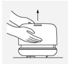
Remove the body cover when it is not locked
