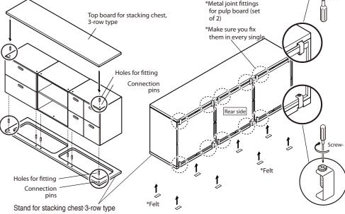
\*6 connection pins are used for the 3-row type and 8 pins for the 4-row type.
