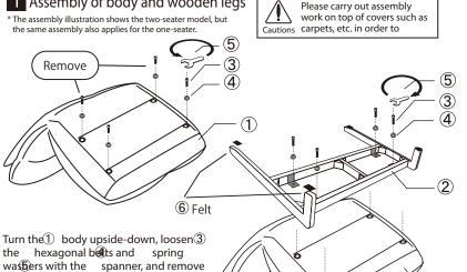
the hexagonal bots and spring washers with the spanner, and remove these from the bodv.
