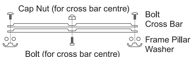
\* Lay cross bars with each other in the direction depicted above. Insert the bolt from the flat side, and loosely tighten cap nut at the indented side. There is no difference between top and bottom sides of the cross bar.
