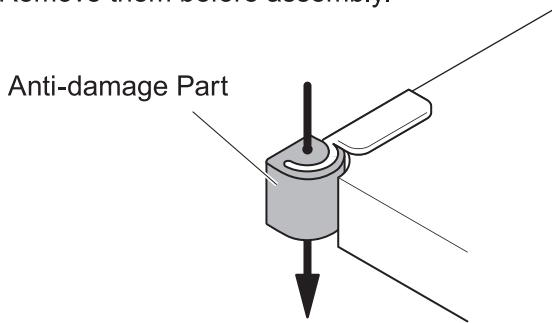
\* Push the part down using a flat-blade screw driver.
