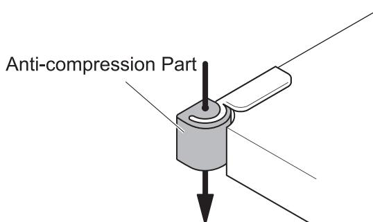
\* Press down against the part using a flat head screwdriver, etc. to remove it.
