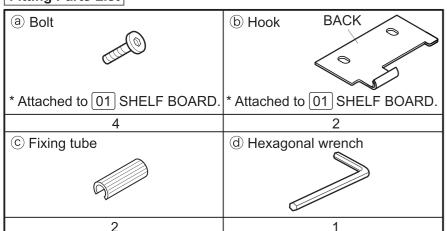
Place a rug/sheet where the product will be assembled. Remove a bolts and b hooks from the reverse of 01 shelf board using @ hexagonal wrench, and reattach as shown in the figure below. Install gently so that (b) hook moves a little.
